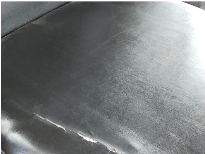
23: Seat Base Cover osf Torn Over 3mm
