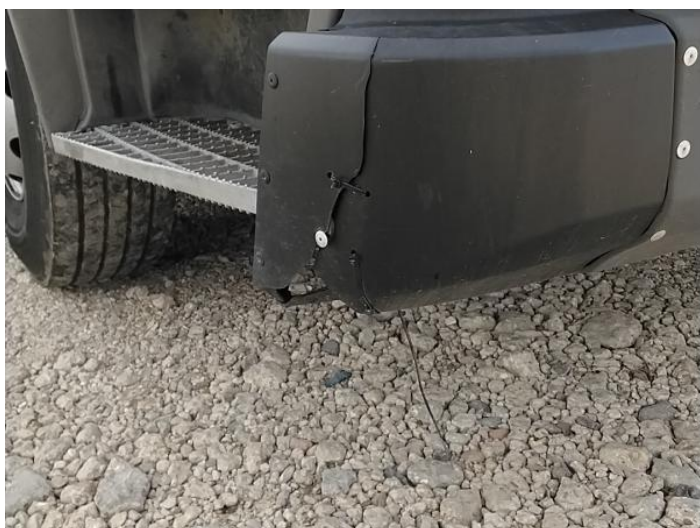
1: Bumper Front Moulding Broken Replace
