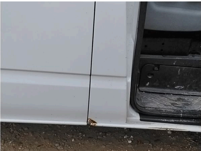
13: B Post os Rusted Over 5mm
