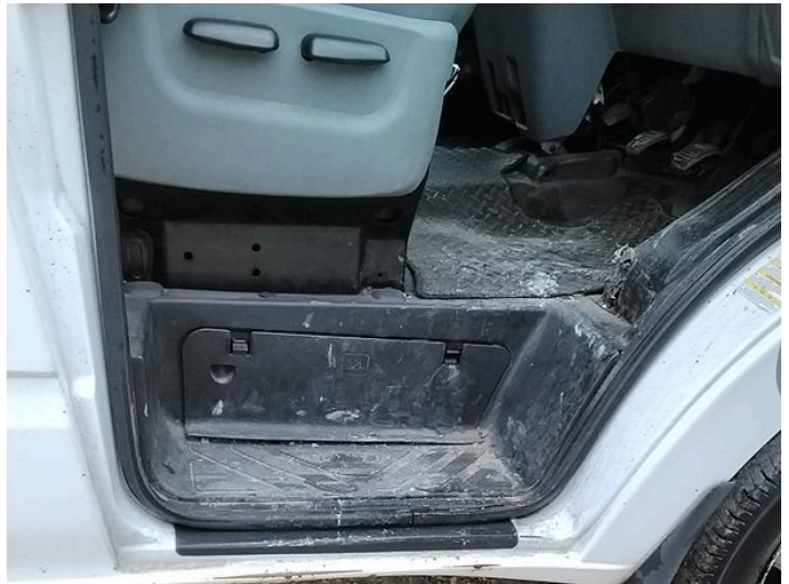
12: Sill os Scratched Over 25mm Thru Paint
